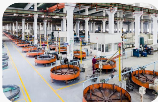
PC Steel Bar Production Line
